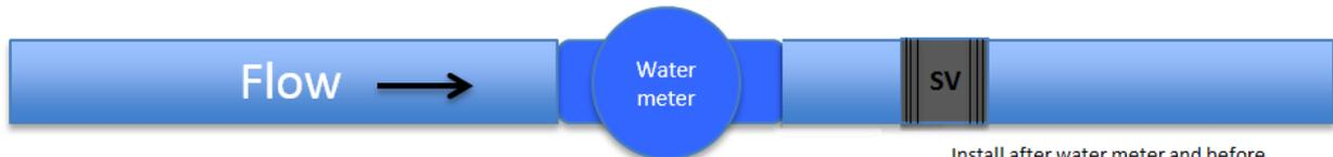
Install after water meter and before pressure reducer or booster pump. Soon after the backflow preventer is usually a good place.
